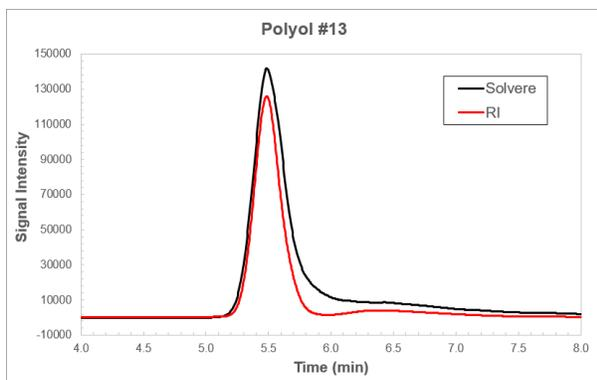
**Figure 3. Overlay of a RI-detected chromatogram and a Solvere-detected chromatogram of a 100% higher MW oxide.**
