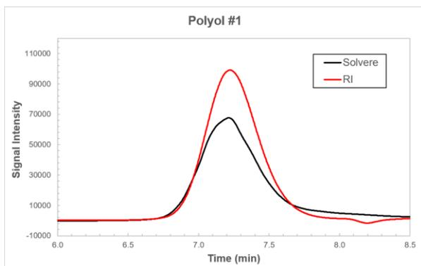
**Figure 2. Overlay of a RI-detected chromatogram and a Solvere-detected chromatogram of a polyol containing 85% of the higher MW oxide.**
