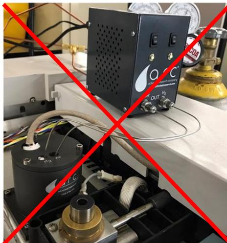
**Figure 2.** Improperly placed EFC
