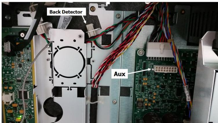
**Figure 5.** Heater connection to back detector port on Agilent 7890 GC (electronics located behind plastic panel on detector side of GC).
