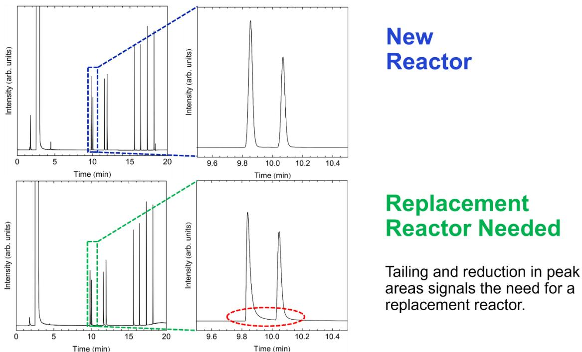
**Figure 1 | Polyarc Reactor Replacement.** Exposure of the Polyarc to silicon or ambient conditions while hot can cause significant peak tailing.
