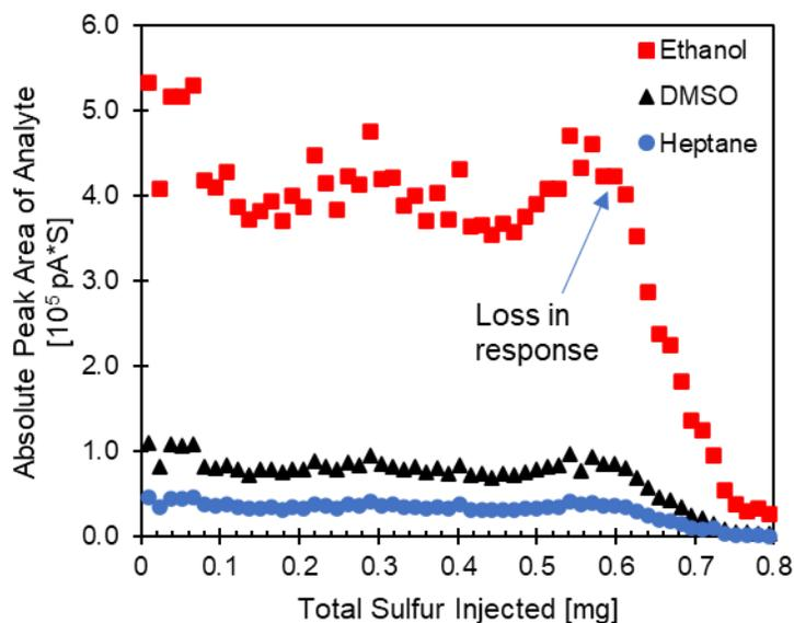
**Figure 2 | Deactivation of the Polyarc from Sulfur Exposure.** The Polyarc reactor can handle a cumulative amount of 0.6 mg of sulfur before showing signs of deactivation for higher concentration analytes first. Injections were for samples with 14 wt% S and 0.1  $\mu$ L splitless injection.
