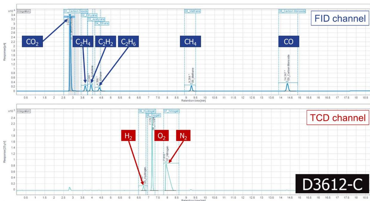
**Figure 2.** D3612-C chromatogram with Polyarc
