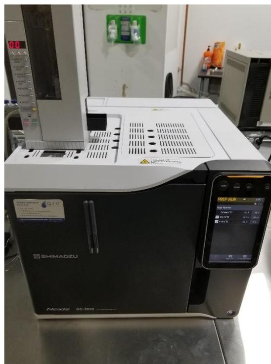
**Figure 1.** Polyarc installed on a Shimadzu GC 2030
