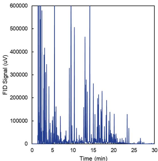
**Figure 2.** GC/FID Gasoline results
