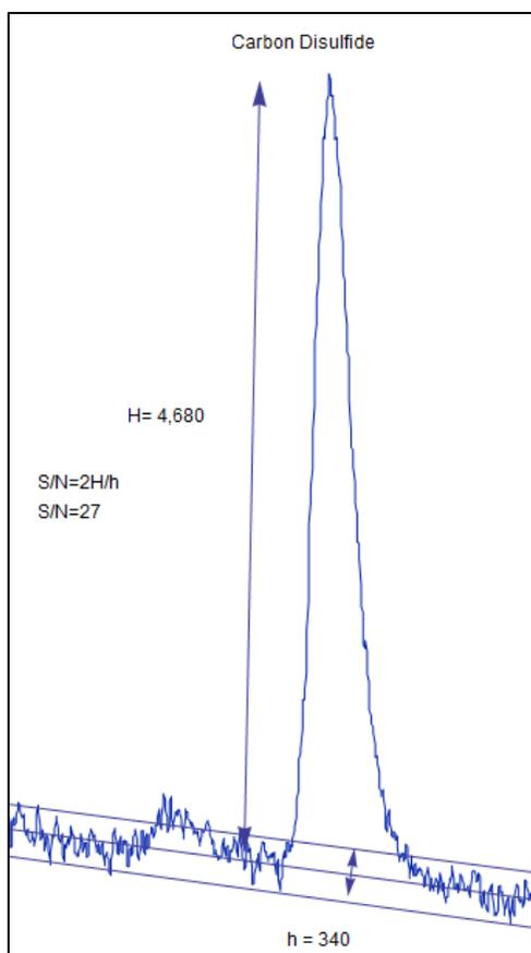
**Figure 3.** Signal-to-noise determination for the analysis of 1.24 ppm CS<sub>2</sub> in 1-propanol using the Polyarc System.
