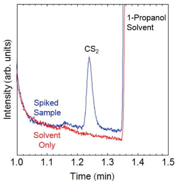
**Figure 2.** Polyarc/FID chromatogram for the analysis of 1.24 mg/kg CS<sub>2</sub> in 1-propanol (blue) and a solvent-only blank (red).
