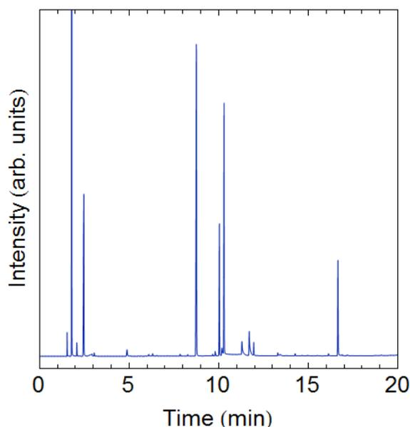
**Figure 2.** Chromatogram of a commercial coating using the Polyarc System.
