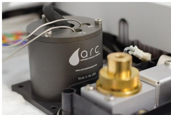
Figure 1. Polyarc System installed in the back detector position next to an FID on an Agilent 7890 GC.
