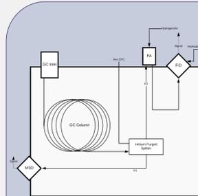
$$S = \frac{F_{Polyarc}}{F_{MS}} = \frac{r_{R2}^4 (P_{split}^2 - P_{Polyarc}^2)}{r_{R1}^4 (P_{split}^2)}$$
