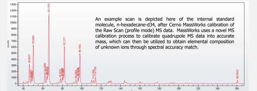
An example scan is depicted here of the internal standard molecule, n-hexadecane-d34, after Cerno MassWorks calibration of the Raw Scan (profile mode) MS data. MassWorks uses a novel MS calibration process to calibrate quadrupole MS data into accurate mass, which can then be utilized to obtain elemental composition of unknown ions through spectral accuracy match.
