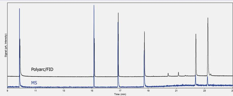
Matching retention times of the MS and Polyarc/FID signals allow for simultaneous identification and quantification. The final two peaks are Tinuvin 328 and Erucamide, and their low signals relative to the other peaks can be observed. This illustrates showing the variation in MS response by compound.
