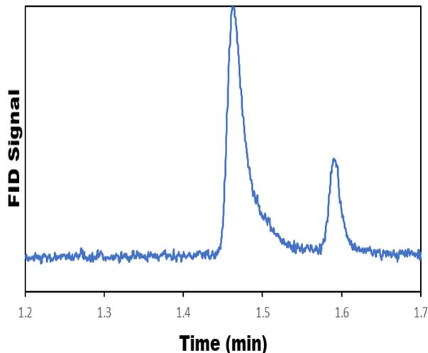
**Figure 2.** Polyarc/FID chromatogram for the analysis of 1.18 mg/kg formaldehyde in HPLC water with a methanol stabilizer using the Polyarc system. (Methanol retention time 1.48; formaldehyde retention time 1.59 minutes)
