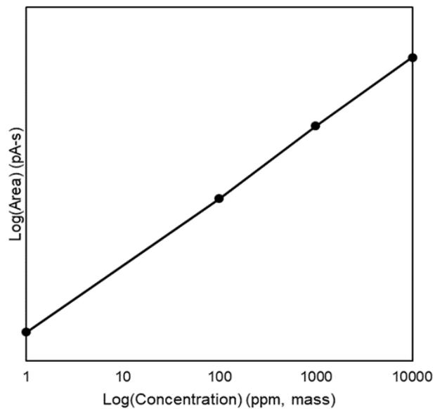
**Figure 3.** Linearity of formaldehyde via Polyarc system. Linear range of over four orders of magnitude.
