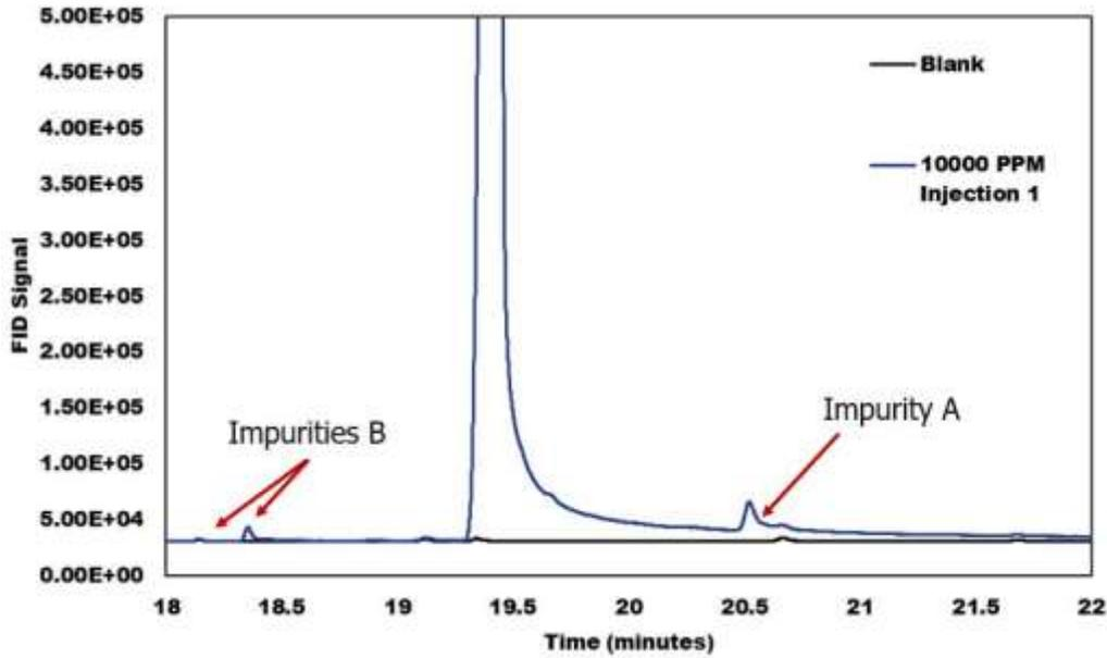
**Figure 3.** Polyarc/FID chromatogram of CBD peak with impurities A and B at minute 20.5 and 18.4 respectively.
