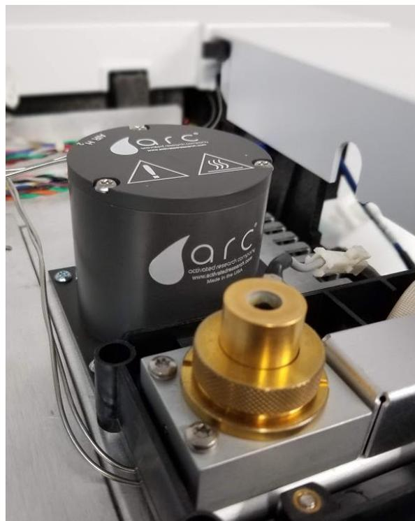
**Figure 1.** Polyarc Ultra on an Agilent 7890 GC.
