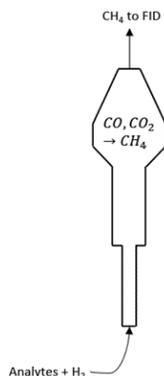
**Figure 1.** Schematic of the Jetanizer
