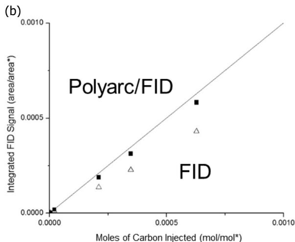
**Figure 6.** Polyarc/FID and FID responses to (a) MeOH and (b) MTBE normalized by the response of toluene. Solid line is the diagonal.
