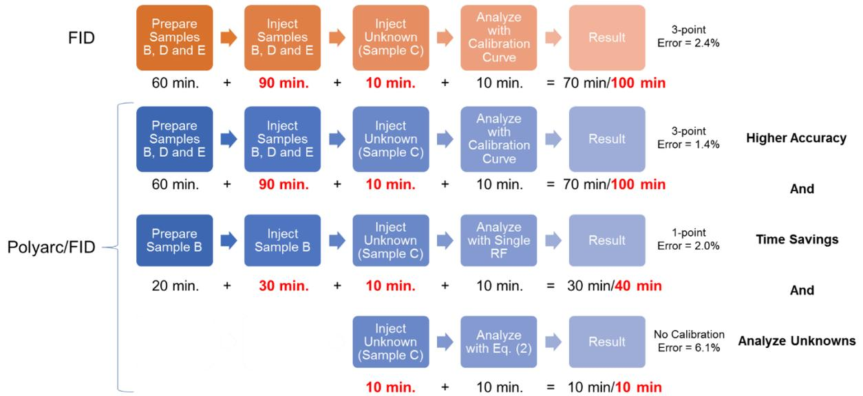
**Figure 8.** Workflow comparison of FID (orange) and Polyarc/FID (blue; from top to bottom correspond to methods (a), (b) and (c) from the text) analysis of sample C. Personnel and instrument time requirements are shown in black and red, respectively.
