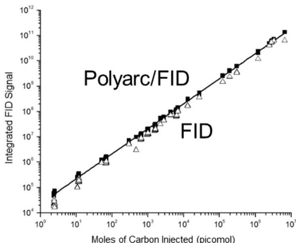
**Figure 3.** Polyarc/FID (solid squares) and FID (open triangles) response to alcohols, ethers and toluene in samples A through G as a function of the amount of carbon injected. Linear regression (line) of Polyarc/FID response gives a slope of 21051, an intercept of  $-3 \cdot 10^7$  and an  $R^2$  of 0.9986.
