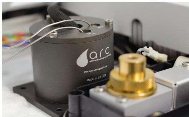
**Figure 1.** Polyarc System installed in the back detector position next to an FID on an Agilent 7890 GC.
