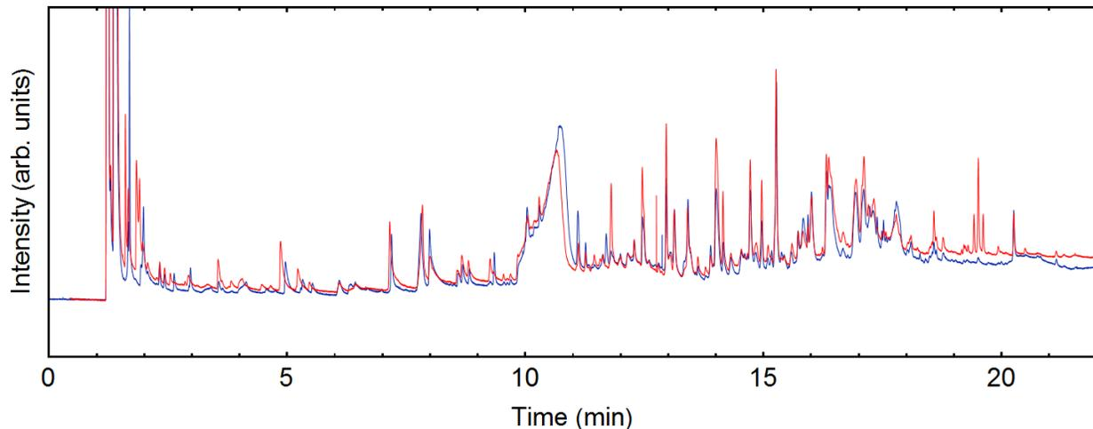
**Figure 2. Polyarc/FID Chromatogram of light lager (blue) and an IPA (red).**
