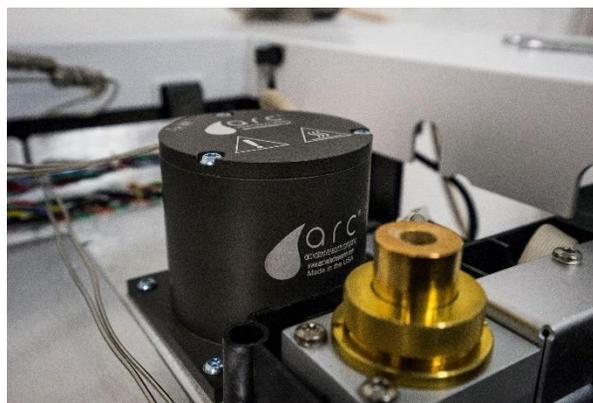
**Figure 1.** Polyarc System on an Agilent 7890 GC.
