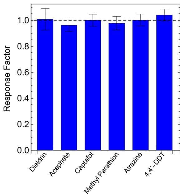
**Figure 4.** Response factors obtained for six pesticides analyzed with the Polyarc™ reactor
