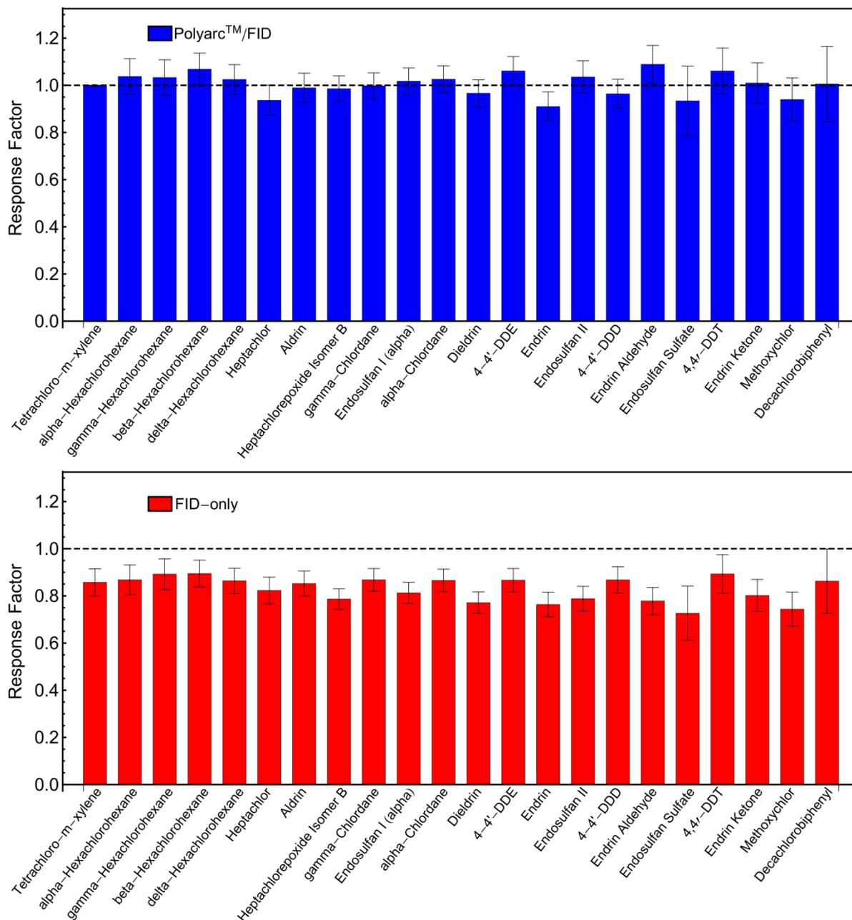
**Figure 3.** Response factors obtained for a 22-component organochlorine pesticide mixture (200 µg/mL in hexane:toluene 1:1) using the Polyarc™ reactor (top) and FID-only (bottom).
