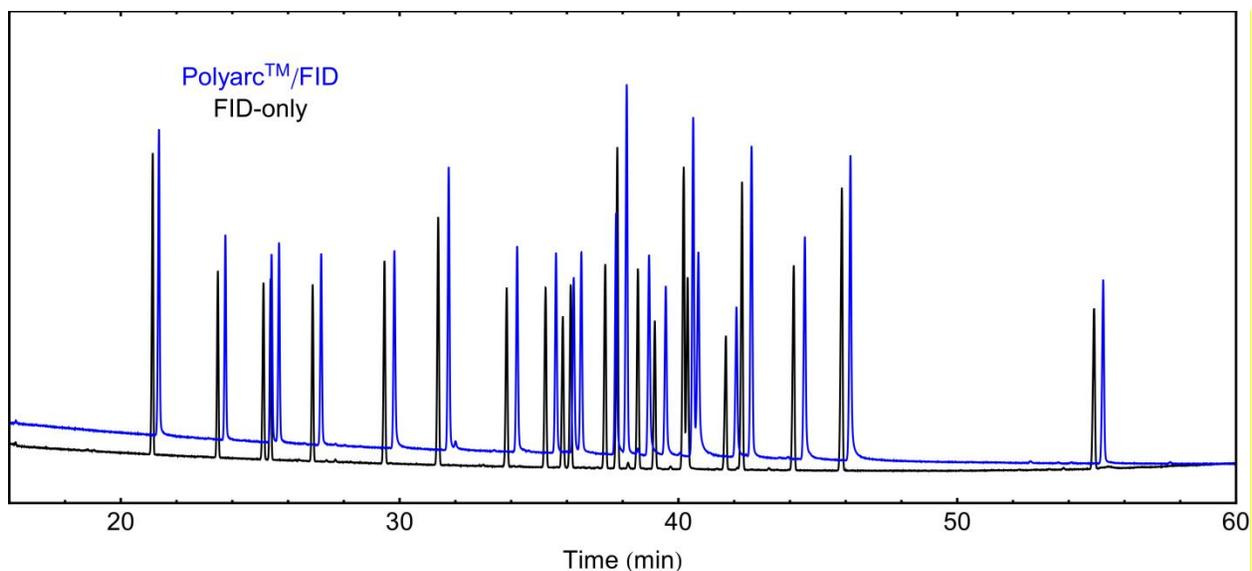
**Figure 1.** Comparison between the chromatograms obtained for a 22-component organochlorine pesticide test mixture using the Polyarc™/FID and FID-only.
